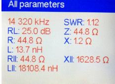
Today I setup the tripod and antenna in an open area away from the house and used Dave NY5A's antenna analyzer. It was resonant at 13.937. I trimmed it back a little at a time and got it 1.12:1 right where I like to talk and below 2:1 across my band plan.
